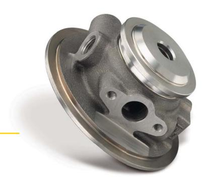
The bearing (or center) housing accommodates the seals and bearing elements of the turbocharger. The cold- and hot-side housings are attached to the bearing housing, while the turbine shaft run centrally through them both.
